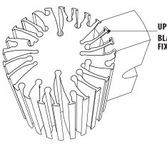
UPWARDS FACING LED = BLACK HEATSINK VISIBLE IN FIXING BLOCK
